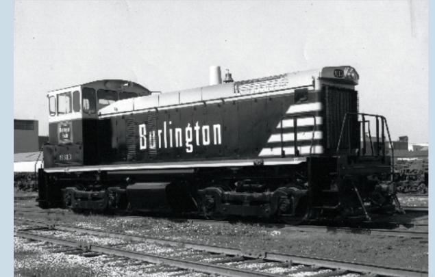
The SW1000 introduced a new cab design and higher-level running boards. *EMD*
