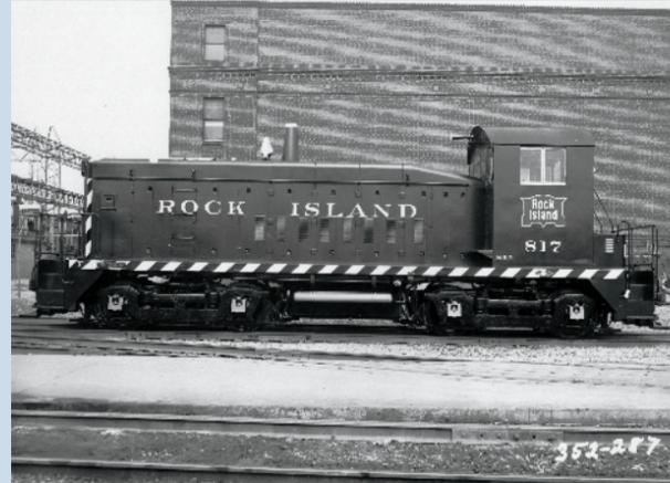
Rock Island No. 817 is an SW8, with a single stack and eight louvered doors on the hood. *EMD*
