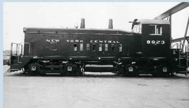
The SW9 has two exhaust stacks and eight louvered hood doors, but lacks the upper set of louvers found on the SW7. *EMD*
