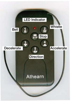
The 12-volt transmitter battery # A23-12, is available at any electronics or office supply store.
