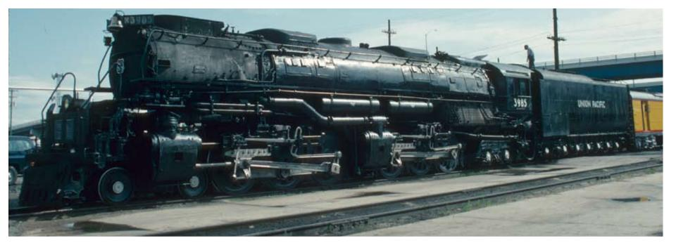
nized locomotives in the world. In 1936, the first group of locomotives with the 4-6-6-4 wheel arrangement was delivered to the Union Pacific Railroad. They were an immediate success and their roster grew to number 105 locomotives on the Union Pacific alone. This new wheel arrangement was given the name "CHALLENGER". While the origin of the name is unclear, it proved to be an apt moniker.
