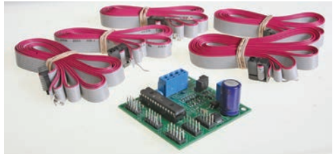
Automatic Block Signaling (ABS) Master NJ International. Operates with any control system (DC or DCC). Provides single track uni-directional signal control. Each BlockMaster can control up to 4 three aspect LED type signals via optical sensors. Unit requires 7-18 volts, AC or DC 300ma. 525-8005 Reg. Price: $139.99 Sale: $119.98
