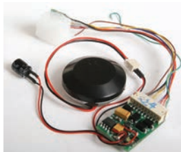
HO Drop-In Sound & Control DCC Decoder - Preferred Sound MRC. Drop in with NMRA 8-pin plug. F1-F18 functions. Includes one prime mover sound, two bells and four horns. Comes with speakers. 500-1618 Heavy/Large Steam Locomotive Sounds Reg. Price: $72.98 Sale: $58.98
