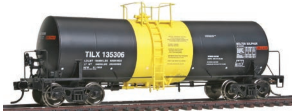
WalthersProto 40' Trinity 14,000-Gallon Molten Sulfur Tank Car Trinity Industries Leasing TILX #135306 920-100023
