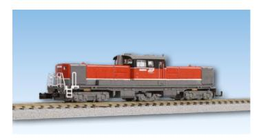
The DD51 is a B2B hydraulic diesel locomotive. A total of 649 locomotives were manufactured by Kawasaki Saryo, Hitachi and Mitsubishi. The loco was used for both freight and passenger trains.
