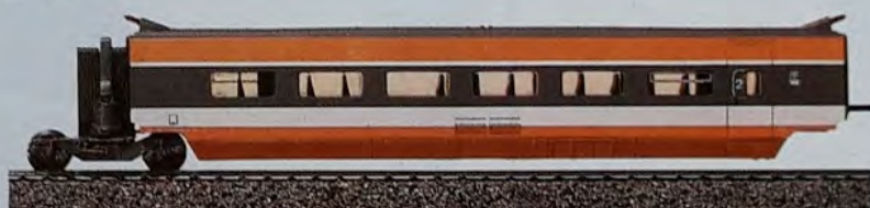
20 1094 - Rimorchiata intermedia TGV di 2° classe, R5-R6-R7. Second class TGV coach of SNCF.
