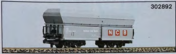
302892 'NCB' coal-hopper wagon with operating doors.
