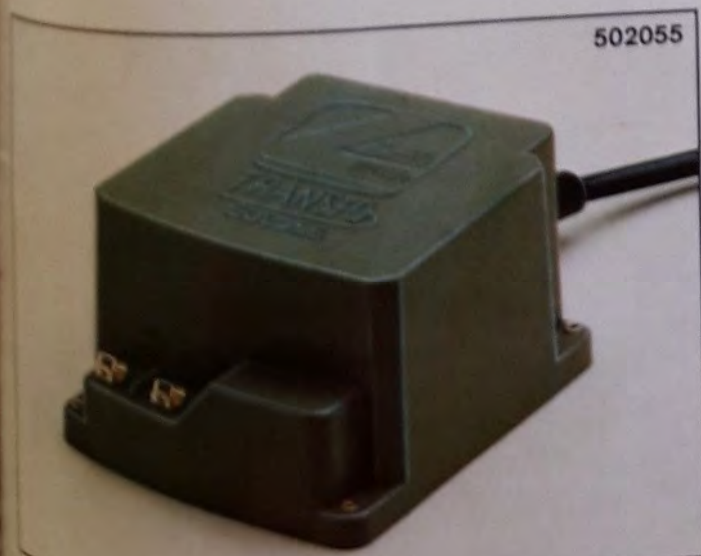
502055 Transformer for electromagnetic devices. Input 220V 50-60 Hz AC. Output 10V AC. Power 7VA.
