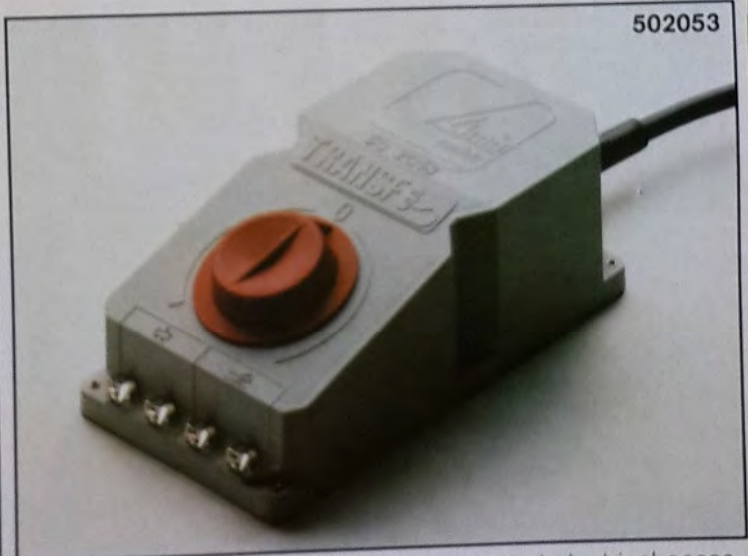
502053 Transformer for two trains, points and electrical accessories. Input 220V. Output 0-12V at 0.7VA DC. AC output 14V at 0.5A.
