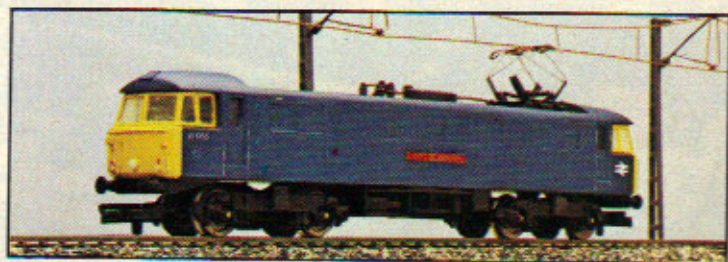
205125MG BR Class 87 Electric Locomotive No. 87005, "City of London", Suitable for operating with or without Catenary system.
