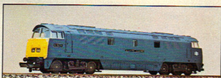
205122MG BR Class 52 'Western' Diesel-Hydraulic Locomotive. No. D1071 "Western Renown".
