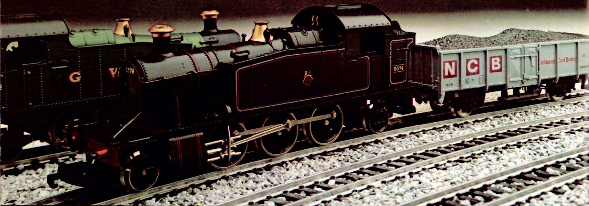
205110/1 One of G.W.R.'s Standard Tank locomotives for cross country and branch line passenger works. The 45 xx Class was designed by G.J. Churchward and 175 were built at Swindon Works between 1906-1929. These small Prairie tanks weighed 57 tons, produced a pressure of 200 lbs and had tractive effort of 21250 lbs superheated.
