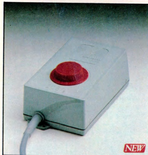
502057 Transformer for 2 trains, points and electrical accessories. Input 220 V. DC Output 0-12V at 0.7A. AC output 14V at 0.5A. Protected against short circuits by thermal cutout.
