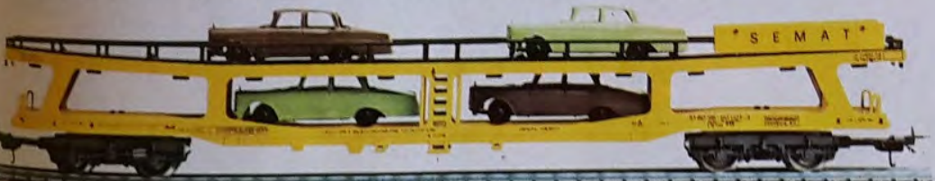
600942 Spanish Semat car transporter wagon with terminal for automatic unloading of cars.
