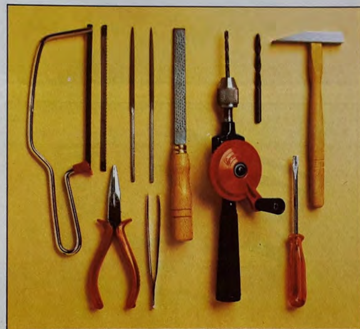
60 0011 The Lima Tool Set contains the basic tools you will need to make your layout: a hacksaw (with one blade for metal and one for wood), two fine files, one rasp, pliers, tweezers, a hand drill (with extra bit), a screwdriver and a hammer.
