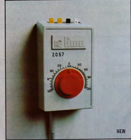
502057 Transformer for 2 trains, points and electrical accessories. Input 220 V. DC Output 0-12V at 0.7A. AC output 14V at 0.5A. Protected against short circuits by thermal cutout. NEW
