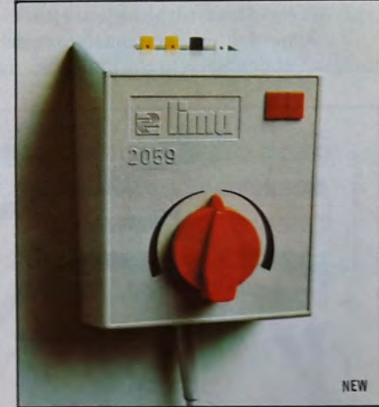
502059 Transformer for several trains, points and accessories. 220V input. DC output 0-15 at 2A. AC output 14 V at 1.2A. Protected against short circuits by thermal cutout. NEW
