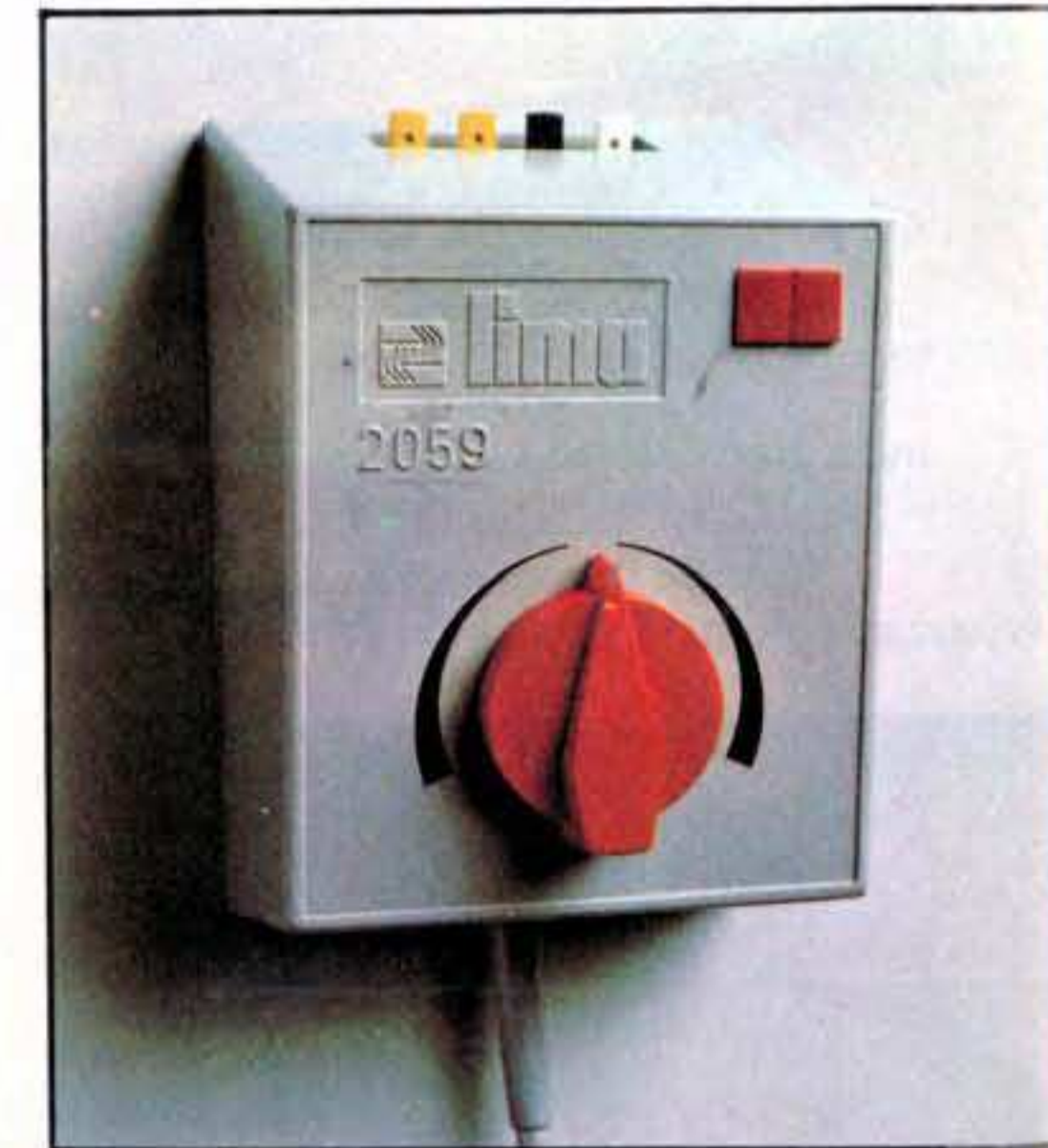
502059 Transformer for several trains, points and accessories. 220V input. DC output 0-15 at 2A. AC output 14 V at 1.2A. Protected against short circuits by thermal cutout.
