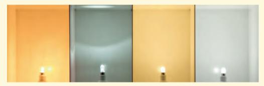
The comparison photo illustrates what makes a good LED: on the left the conventional FALLER light bulb, to the right of it an LED with particularly uneven lighting, as offered in stores.
