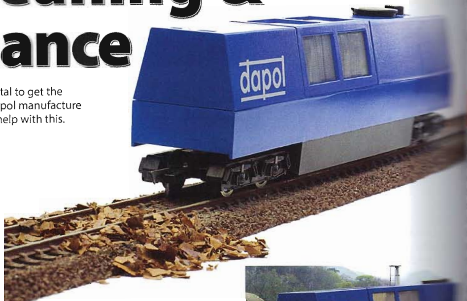
B800 The OO/HO gauge Dapol motorised track cleaner with 5 in one functionality that gently scrubs, vacuums, applies a special cleaning fluid, polishes and sweeps all in one. The unit runs on both DC and DCC layouts thanks to the 8 pin DCC socket included. To operate, the unit has to be hauled or pushed with a locomotive as the onboard motor powers the cleaning and vacuuming functions only. The cleaner also features NEM pockets, complete with scrubbing and 3 polishing pads, plus DCC ready and with a suitable chip fitted enabling all the functions to be operated independently.
