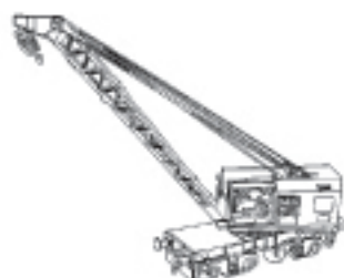
C028: 15t Diesel Crane
