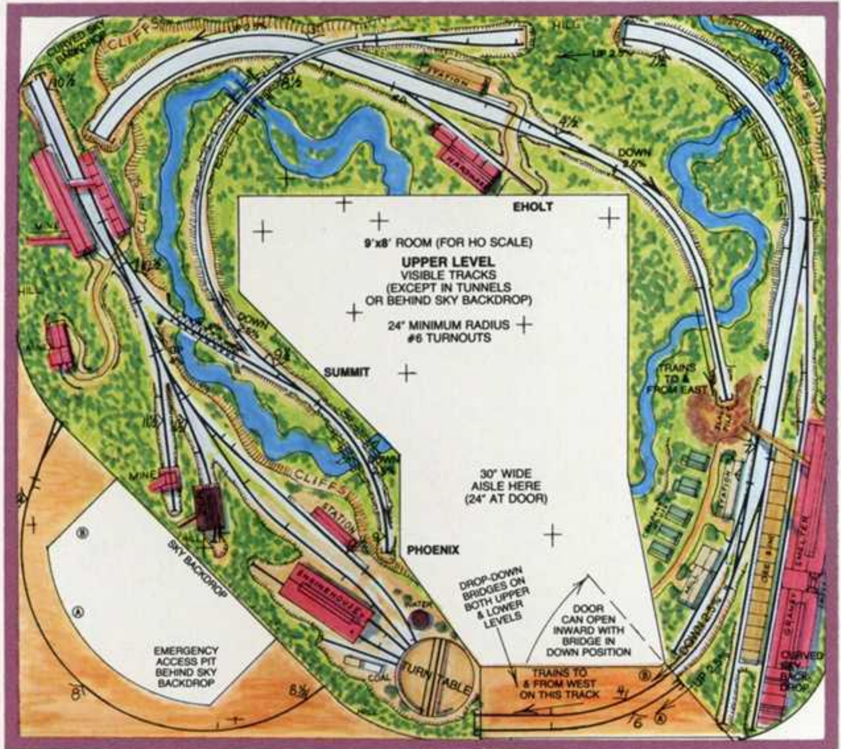
An example of how you can have mainline model railroading with 24 inch minimum radius curves in a spare room as small as 9 x 8 ft. This plan includes a lower level staging yard for 12 car trains. It's from THE BEST OF MODEL RAILROADING Magazine's Track Plan Book . Order Book #0100-12109. Photo courtesy Model Railroading magazine.
