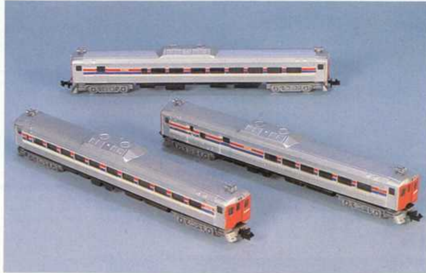
TOP RDC-2 Amtrak, note extra baggage door at left end of RDC Middle RDC-3, Amtrak, note almost 1/2 car is baggage/freight Bottom RDC-1, Amtrak, Full passenger version, no extra space for baggage
