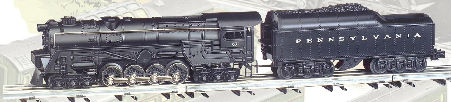
STEAM POWER 6-8-6 PRR S-2 TURBINE
