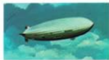
93. Hindenburg Length 604 ft. Engines Four 1,320-hp. diesels Diameter 125 ft. Payload 7,062,500 Fuel Load 2,000 tons Speed 80 knots Rate of Hydrogen Scale 1:280
