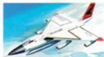
98. B-58 Hustler Length 96 ft. 9 in. Speed 1,524 m.p.h. Wingspan 56 ft. 10 in. Scale 1:260 Height 29 ft.
