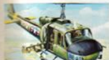
94. Bell UH-1H Iroquois Length 39 ft. 4 in. Speed 180 m.p.h. Rotor Diameter 44 ft. Scale 1:250 Height 12 ft. 4 1/2 in.
