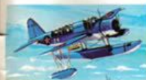
93. Kingfisher Length 33 ft. 7 in. Speed 171 m.p.h. Wingspan 25 ft. 2 1/2 in. Scale 1:160 Height 14 ft. 8 in.
