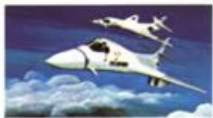
95. North American Rockwell B-1 Length 150 ft. Engines Four GE turbofans Wingspan 156 ft. Swept 78 ft. Twice speed of sound Forward 135 ft. Scale 1:400
