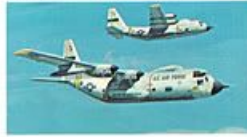
88. Lockheed C-130 Hercules Height ..... 38 ft. 4 in. Length ..... 97 ft. 9 in. Speed ..... 384 m.p.h. Wingspan ..... 132 ft. 7 in. Scale ..... 1:400
