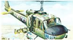
69. Bell UH-1B Iroquois Height ..... 32 ft. 4 1/2 in. Length ..... 39 ft. 4 in. Speed ..... 180 m.p.h. Rotor Diameter 44 ft. Scale ..... 1:200
