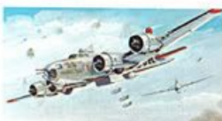
6. B-17 Flying Fortress Length ..... 74 ft. 4 in. Wingspan ..... 103 ft. 9 in. Height ..... 19 ft. 1 in. Speed ..... 300 m.p.h. Scale ..... 1:250
