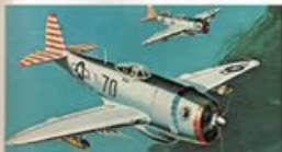
92. P-47D Thunderbolt Height ..... 14 ft. 2 in. Length ..... 36 ft. 1 in. Wingspan ..... 40 ft. 9 in. Speed ..... 429 m.p.h. Scale ..... 1:160
