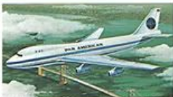
35. Boeing 747 Height ..... 63 ft. 5 in. Length ..... 231 ft. 10 in. Speed ..... 615 m.p.h. Wingspan ..... 195 ft. 8 in. Scale ..... 1:665
