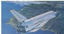
07. Space Shuttle Height ..... 56 ft. 8 in. Length ..... 122 ft. 2 1/2 in. Speed ..... 17,450 m.p.h. Wingspan ..... 78 ft. 1/2 in. Scale ..... 1:500
