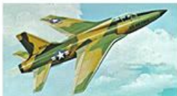
96. F-105 Thunderchief Height ..... 19 ft. 8 in. Length ..... 64 ft. 4 in. Speed ..... 1390 m.p.h. Wingspan ..... 34 ft. 11 in. Scale ..... 1:240
