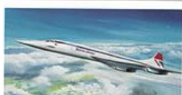
05. Concorde Length ..... 203 ft. 9 in. Wingspan ..... 83 ft. 10 in. Height ..... 37 ft. 1 in. Speed ..... Mach 2.0 Scale ..... 1:600
