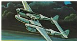
97. P-38 Lightning Height ..... 12 ft. 10 in. Length ..... 37 ft. 10 in. Speed ..... 390 m.p.h. Wingspan ..... 52 ft. Scale ..... 1:160
