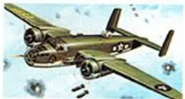
14. B-25 Mitchell Length ..... 53 ft. 5 1/2 in. Wingspan ..... 62 ft. 7 in. Height ..... 16 ft. 4 in. Speed ..... 303 m.p.h. Scale ..... 1:190
