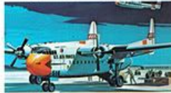
45. C-119 Flying Box Car Height ..... 26 ft. 3 in. Length ..... 86 ft. 6 in. Speed ..... 296 m.p.h. Wingspan ..... 109 ft. 3 in. Scale ..... 1:340
