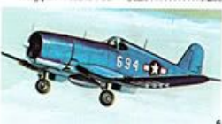
15. F-4U Corsair Length ..... 33 ft. 8 1/2 in. Wingspan 40 ft. 11 1/2 in. Height ..... 14 ft. 9 1/2 in. Speed ..... 425 m.p.h. Scale ..... 1:160
