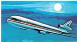
40. Douglas DC-10 Height ..... 57 ft. 3 1/2 in. Length ..... 179 ft. 3 1/2 in. Speed ..... 561 m.p.h. Wingspan ..... 155 ft. 5 in. Scale ..... 1:655
