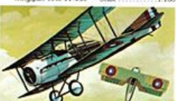
18. Spad XIII Length ..... 20 ft. 8 in. Wingspan ..... 26 ft. 11 in. Height ..... 7 ft. 11 1/2 in. Speed ..... 130 m.p.h. Scale ..... 1:100
