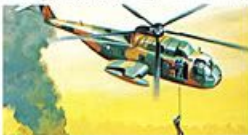
38. Jolly Green Giant Height ..... 16 ft. 1 in. Length ..... 57 ft. 3 in. Speed ..... 303 m.p.h. Rotor Diameter 62 ft. Scale ..... 1:260
