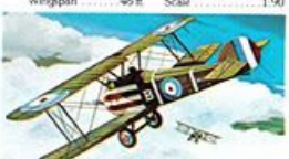
20. Sopwith Camel Length ..... 18 ft. 6 in. Wingspan ..... 27 ft. Height ..... 8 ft. 6 in. Speed ..... 121 m.p.h. Scale ..... 1:90
