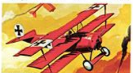
17. Fokker DR-1 Length ..... 19 ft. Wingspan ..... 23 ft. 7 in. Height ..... 9 ft. 9 in. Speed ..... 115 m.p.h. Scale ..... 1:90
