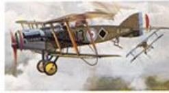
06. Bristol F2B Fighter Height ..... 9 ft. 9 in. Length ..... 25 ft. 10 in. Speed ..... 113 m.p.h. Wingspan ..... 39 ft. 3 in. Scale ..... 1:120
