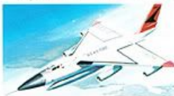
65. B-58 Hustler Height ..... 29 ft. Length ..... 96 ft. 9 in. Speed ..... 1324 m.p.h. Wingspan ..... 56 ft. 10 in. Scale ..... 1:260
