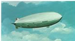
93. Hindenburg Engines Length ..... 804 ft. Four 1320 h.p. diesels Diameter ..... 135 ft. Speed ..... 80 knots Payload ..... 7,062,100 cubic ft. of hydrogen Scale ..... 1:180
