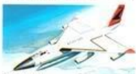
65. B-58 Hustler Height 29 ft. Length 96 ft. 9 in. Speed 1324 m.p.h. Wingspan 56 ft. 10 in. Scale 1:200
