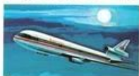
40. Douglas DC-10 Height 57 ft. 3 1/2 in. Length 179 ft. 3 1/2 in. Speed 560 m.p.h. Wingspan 150 ft. 5 in. Scale 1:600
