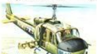
66. Bell UH-1H Helicopter Height 12 ft. 4 1/2 in. Length 39 ft. 4 in. Rotor Diameter 44 ft. Speed 180 m.p.h. Scale 1:200
