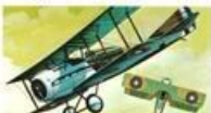
18. Spad XIII Height 7 h. 11 in. Length 20 h. 8 in. Speed 130 m.p.h. Wingspan 26 h. 11 in. Scale 1:150
