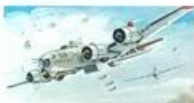
6. B-17 Flying Fortress Height 19 h. 1 in. Length 74 h. 4 in. Speed 300 m.p.h. Wingspan 103 h. 9 in. Scale 1:250
