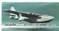
94. Hughes Hercules HHC-1 Engines Eight 2000 h.p. Length 218 ft. 6 in. Speed 218 m.p.h. (sea level) Wingspan 320 ft. Scale 1:850 Height 79 ft. 3 in.
