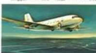
72. Douglas DC-3 Height 34 ft. 11 in. Length 64 ft. 6 in. Speed 167 m.p.h. Wingspan 90 ft. Scale 1:240
