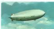
93. Hindenburg Engines 804 ft. Length 135 ft. Four 1320 h.p. diesel Diameter 115 ft. Speed 80 knots Payload 7,062 lbs. Scale 1:180 cubic ft. of hydrogen
