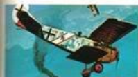
33. Fokker D-VII Height 95.2 in. Length 22 ft. 9 in. Speed 135 m.p.h. Wingspan 29 ft. 3 1/2 in. Scale 1:250
