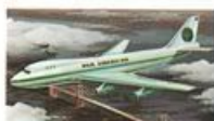
35. Boeing 747 Height 63 ft. 5 in. Length 231 ft. 10 in. Speed 453 m.p.h. Wingspan 195 ft. 8 in. Scale 1:600
