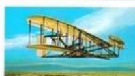
37. Kitty Hawk Height 7 ft. 2 in. Length 35 ft. 6 in. Speed 42 m.p.h. Wingspan 40 ft. 4 in. Scale 1:100
