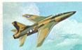
06. F-105 Thunderchief Height ..... 19 ft. 8 in. Length ..... 42 ft. 4 in. Speed ..... 1390 m.p.h. Wingspan ..... 34 ft. 11 in. Scale ..... 1:240
