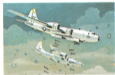
64. Boeing B-29 Superfortress Height ..... 29 ft. Length ..... 98 ft. 2 in. Speed ..... 388 m.p.h. Wingspan ..... 141 ft. 5 in. Scale ..... 1:380
