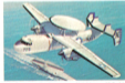
77. Curtiss Wright Height ..... 18 ft. 4 in. Length ..... 50 ft. 4 in. Speed ..... 370 m.p.h. Wingspan ..... 80 ft. 7 in. Scale ..... 1:210
