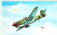
1. P-40 Flying Tiger Height ..... 12 ft. 4 in. Length ..... 27 ft. 4 in. Wingspan ..... 37 ft. 4 in. Speed ..... 303 m.p.h. Scale ..... 1/100
