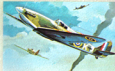
7. British Spitfire Height ..... 11 ft. 5 in. Length ..... 29 ft. 11 in. Wingspan ..... 36 ft. 10 in. Speed ..... 362 m.p.h. Scale ..... 1/140
