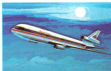
40. Douglas DC-10 Height ..... 57 ft. 3 1/2 in. Length ..... 174 ft. 3 1/2 in. Speed ..... 561 m.p.h. Wingspan 165 ft. 8 in.
