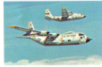
80. Lockheed C-130 Hercules Height ..... 28 ft. 4 in. Length ..... 132 ft. 7 in. Speed ..... 384 m.p.h. Wingspan ..... 132 ft. 7 in. Scale ..... 1:400
