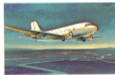
72. Douglas DC-3 Height ..... 38 ft. 11 in. Length ..... 64 ft. 8 in. Speed ..... 327 m.p.h. Wingspan ..... 85 ft. Scale ..... 1:240
