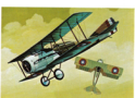
18. Speed King Length ..... 20 ft. 8 in. Wingspan 26 ft. 11 in. Height ..... 7 ft. 11 1/2 in. Speed ..... 130 m.p.h. Scale ..... 1:100
