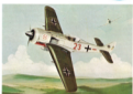
63. Focke-Wulf 190 Length ... 27 ft. 6 in. Wingspan 24 ft. 6 in. Height ... 13 ft. Speed ... 405 m.p.h. Scale ... 1:140
