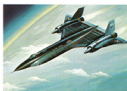
26. YF-12A Lockheed Height ... 18 ft. 6 in. Length ... 107 ft. 5 in. Wingspan ... 55 ft. 7 in. Speed ... 1,960 m.p.h. Scale ... 1:140
