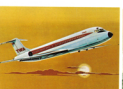
23. Douglas DC-9 Length ..... 104 ft. 4 in. Wingspan ..... 89 ft. 5 in. Height ..... 27 ft. 6 in. Speed ..... 561 m.p.h. Scale ..... 1:290
