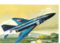
24. F-4E Phantom Length ..... 58 ft. 3 in. Wingspan 38 ft. 5 in. Height ..... 16 ft. 3 in. Speed ..... 1,584 m.p.h. Scale ..... 1:25
