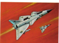
41. Saab A37 Viggen Length 53 ft. 5 1/2 in. Wingspan 34 ft. 9 1/2 in. Height ..... 16 ft. 4 1/2 in. Speed Over 1,400 m.p.h. Scale ..... 1:125
