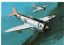
32. P-47D Thunderbolt Height ... 14 ft. 2 in. Length ... 36 ft. 1 in. Wingspan ... 40 ft. 9 in. Speed ... 429 m.p.h. Scale ... 1:50
