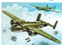
14. B-25 Mitchell Length ..... 53 ft. 5 1/2 in. Wingspan ..... 67 ft. 7 in. Height ..... 16 ft. 4 1/2 in. Speed ..... 303 m.p.h. Scale ..... 1:190
