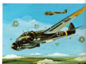
27. Junker Ju-88 Height ... 15 ft. 11 in. Length ... 47 ft. 1 1/2 in. Wingspan ... 65 ft. 10 1/2 in. Speed ... 273 m.p.h. Scale ... 1:170
