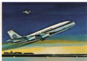
9. Boeing 707 Height . . . 42 ft. Length . . . 144 ft. 6 in. Wingspan . . . 130 ft. 10 in. Speed . . . 571 m.p.h. Scale . . . 1:440
