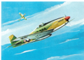
11. P-51 Mustang Height . . . 37 ft. 8 in. Length . . . 32 ft. 3 in. Wingspan . . . 37 ft. Speed . . . 437 m.p.h. Scale . . . 1:150
