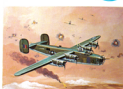
39. B-24D Liberator Length ..... 66 ft. 4 in. Wingspan ..... 133 ft. Height ..... 37 ft. 11 in. Speed ..... 303 m.p.h. Scale ..... 1:340
