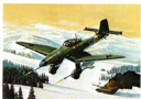
31. Stuka Ju-87G-1 Height ... 17 ft. 9 in. Length ... 35 ft. 5 in. Wingspan ... 49 ft. 2 in. Speed ... 218 m.p.h. Scale ... 1:160
