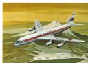
25. Douglas DC-8 Height ... 82 ft. 4 in. Length ... 150 ft. 6 in. Wingspan ... 142 ft. 5 in. Speed ... 580 m.p.h. Scale ... 1:450
