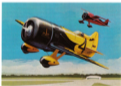
68. See Bee Racer Length ... 15 ft. 3 in. Wingspan 25 ft. 6 in. Height ... 7 ft. 6 in. Speed ... 273 m.p.h. Scale ... 1:90
