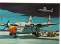
45. C-139 Flying Box Car Length ..... 66 ft. 5 in. Wingspan 109 ft. 3 in. Height ..... 26 ft. 3 in. Speed ..... 296 m.p.h. Scale ..... 1:140
