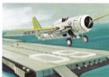
62. Grumman F4F Wildcat Length ... 29 ft. Wingspan ... 38 ft. Height ... 13 ft. Speed ... 331 m.p.h. Scale ... 1:340
