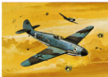
2. Messerschmitt ME-109 Height . . . 7 ft. 8 in. Length . . . 29 ft. 5 in. Wingspan . . . 32 ft. 8 in. Speed . . . 374 m.p.h. Scale . . . 1:140
