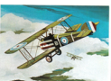
20. Sopwith Camel Length ..... 18 ft. 6 in. Wingspan ..... 28 ft. Height ..... 8 ft. 6 in. Speed ..... 123 m.p.h. Scale ..... 1:90
