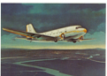
72. Douglas DC-3 Length ... 64 ft. 6 in. Wingspan ... 36 ft. Height ... 16 ft. 11 in. Speed ... 167 m.p.h. Scale ... 1:360
