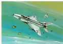
3. Russian MIG 21-C Height . . . 14 ft. 6 in. Length . . . 47 ft. Wingspan . . . 25 ft. Speed . . . 1,320 m.p.h. Scale . . . 1:160
