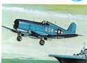
15. F-4U Corsair Length ..... 23 ft. 9 1/2 in. Wingspan 40 ft. 11 1/2 in. Height ..... 14 ft. 9 1/2 in. Speed ..... 425 m.p.h. Scale ..... 1:160
