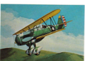
42. Curtiss P4E Hawk Length ..... 23 ft. 3 in. Wingspan ..... 51 ft. 5 in. Height ..... 10 ft. 3 in. Speed ..... 197.8 m.p.h. Scale ..... 1:100
