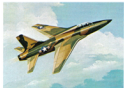
10. F-105 Thunderchief Height . . . 19 ft. 8 in. Length . . . 64 ft. 4 in. Wingspan . . . 34 ft. 11 in. Speed . . . 1,390 m.p.h. Scale . . . 1:240
