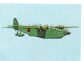
48. S56A Flying Boat Length ..... 57 ft. 4 in. Wingspan 124 ft. 8 in. Height ..... 30 ft. Speed ..... 290 m.p.h. Scale ..... 1:110
