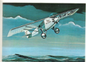
16. Spirit of St. Louis Length ..... 27 ft. 8 in. Wingspan ..... 46 ft. Height ..... 9 ft. 10 in. Speed ..... 124.5 m.p.h. Scale ..... 1:90
