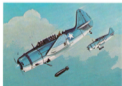
70. Curtis Helldiver Length ... 35 ft. 2 in. Wingspan 49 ft. 7 in. Height ... 14 ft. 9 in. Speed ... 225 m.p.h. Scale ... 1:160
