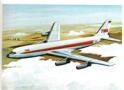
19. Convair 880 Length ..... 129 ft. 4 in. Wingspan ..... 123 ft. Height ..... 36 ft. 4 in. Speed ..... 605 m.p.h. Scale ..... 1:400
