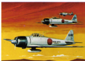
8. Japanese Zero-Zen Height . . . 9 ft. 2 in. Length . . . 29 ft. 9 in. Wingspan . . . 36 ft. 1 in. Speed . . . 346 m.p.h. Scale . . . 1:140
