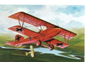
21. Albatross D-III Length ..... 24 ft. Wingspan 29 ft. 7 in. Height ..... 9 ft. 9 1/2 in. Speed ..... 155 m.p.h. Scale ..... 1:110
