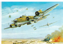
6. B-17 Flying Fortress Height . . . 19 ft. 1 in. Length . . . 74 ft. 4 in. Wingspan . . . 102 ft. 9 in. Speed . . . 300 m.p.h. Scale . . . 1:250
