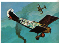
33. Fokker D-VII Height ... 9 ft. 7 in. Length ... 27 ft. 9 in. Wingspan ... 29 ft. 3 1/2 in. Speed ... 116 m.p.h. Scale ... 1:110
