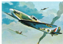
7. British Spitfire Height . . . 11 ft. 5 in. Length . . . 29 ft. 11 in. Wingspan . . . 36 ft. 10 in. Speed . . . 362 m.p.h. Scale . . . 1:140
