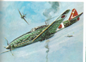
46. Kawasaki Ki-61-II Length ..... 32 ft. 3 in. Wingspan ..... 39 ft. 4 in. Height ..... 12 ft. 1 in. Speed ..... 362 m.p.h. Scale ..... 1:145
