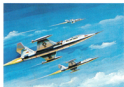
4. F-104 Starfighter Height . . . 13 ft. 6 in. Length . . . 34 ft. 9 in. Wingspan . . . 21 ft. 11 in. Speed . . . 1,450 m.p.h. Scale . . . 1:210
