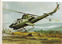
13. Huey Copter AH-1G Length ..... 44 ft. 5 in. Rotor Diameter 44 ft. Height ..... 13 ft. Speed ..... 196 m.p.h. Scale ..... 1:210
