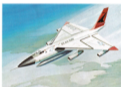
65. S-56 Hurrier Length ... 36 ft. 9 in. Wingspan 56 ft. 10 in. Height ... 29 ft. Speed ... 1304 m.p.h. Scale ... 1:360
