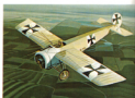
30. Fokker Eindecker Height ... 7 ft. 10 in. Length ... 33 ft. 5 1/2 in. Wingspan ... 32 ft. 9 in. Speed ... 87 1/2 m.p.h. Scale ... 1:110
