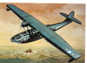
44. PB4Y-2 Catalina Length ..... 65 ft. 2 in. Wingspan ..... 104 ft. Height ..... 20 ft. 2 in. Speed ..... 179 m.p.h. Scale ..... 1:340
