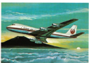
35. Boeing 747 Height ... 63 ft. 5 in. Length ... 231 ft. 10 in. Wingspan ... 195 ft. 8 in. Speed ... 453 m.p.h. Scale ... 1:55
