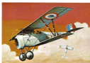
29. Nieuport 17 Height ... 8 ft. Length ... 38 ft. 11 in. Wingspan ... 26 ft. 10 in. Speed ... 107 m.p.h. Scale ... 1:90
