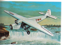
43. Ford Tri-Motor Length ..... 49 ft. 10 in. Wingspan ..... 74 ft. Height ..... 11 ft. 3 in. Speed ..... 130 m.p.h. Scale ..... 1:260
