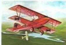
21. Albatross D-III Height ... 9 ft. 9 1/2 in. Length ... 24 ft. Wingspan 29 ft. 7 in. Speed ... 115 m.p.h. Scale ..... 1:110
