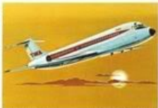
23. Douglas DC-9 Height ... 27 ft. 6 in. Length ... 104 ft. 4 in. Wingspan 89 ft. 5 in. Speed ... 543 m.p.h. Scale ..... 1:190
