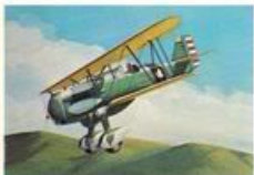
42. Curtiss P-6E Hawk Length ... 23 ft. 2 in. Wingspan 31 ft. 6 in. Height ... 10 ft. 3 in. Speed ... 137.8 m.p.h. Scale ... 1:100
