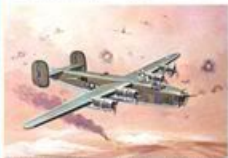
39. B-24D Liberator Length ... 66 ft. 4 in. Wingspan ... 110 ft. Height ... 17 ft. 11 in. Speed ... 323 m.p.h. Scale ... 1:340
