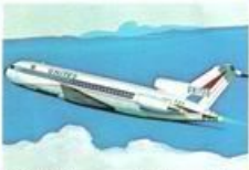
22. Boeing 727 Height ... 34 ft. Length ... 133 ft. 2 in. Wingspan ... 108 ft. Speed ... 605 m.p.h. Scale ..... 1:110
