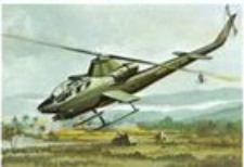
13. Huey Helicopter AH-1G Height ... 13 ft. Length ... 44 ft. 5 in. Rotor Diameter 44 ft. Speed ... 196 m.p.h. Scale ..... 1:210
