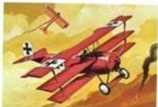
17. Fokker DR-1 Length 19 ft. Wingspan 23 ft. 7 in. Height 9 ft. 9 in. Speed 115 m.p.h. Scale 1:90
