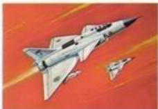
41. Saab A37 Viggen Length ... 51 ft. 5 1/2 in. Wingspan 34 ft. 9 1/4 in. Height ... 18 ft. 4 1/2 in. Speed Over 1,400 m.p.h. Scale ... 1:125
