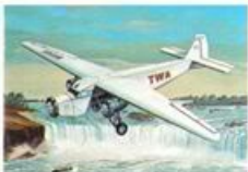
43. Ford Tri-Motor Length ... 49 ft. 10 in. Wingspan ... 74 ft. Height ... 11 ft. 9 in. Speed ... 330 m.p.h. Scale ... 1:260
