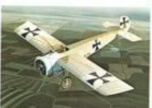
30. Fokker Eindecker Length ... 23 ft. 6 1/2 in. Wingspan ... 32 ft. 8 in. Height ... 7 ft. 10 in. Speed ... 87 1/2 m.p.h. Scale ... 1:110
