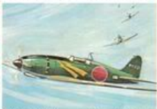
57. Mitsubishi J2M3 Length ... 21 ft. 8 in. Wingspan ... 35 ft. 4 in. Height ... 12 ft. 6 in. Speed ... 374 m.p.h. Scale ... 1:190
