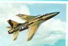
10. F-105 Thunderchief Length 64 ft. 4 in. Wingspan 34 ft. 11 in. Height 19 ft. 8 in. Speed 1,390 m.p.h. Scale 1:240
