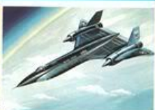
26. YF-12A Lockheed Length ... 107 ft. 5 in. Wingspan ... 55 ft. 7 in. Height ... 18 ft. 6 in. Speed ... 1,980 m.p.h. Scale ... 1:140
