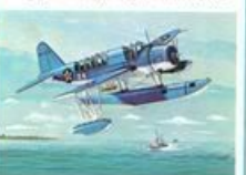
36. Kingfisher Length ... 33 ft. 7 in. Wingspan 35 ft. 10 in. Height ... 14 ft. 6 in. Speed ... 171 m.p.h. Scale ... 1:160
