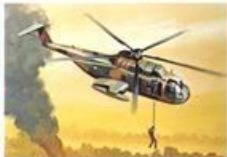
38. Jolly Green Giant Length ... 57 ft. 3 in. Rotor Diameter 62 ft. Height ... 16 ft. 1 in. Speed ... 303 m.p.h. Scale ... 1:200
