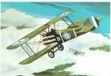
20. Sopwith Camel Height ... 8 ft. 6 in. Length ... 18 ft. 6 in. Wingspan ... 28 ft. Speed ... 121 m.p.h. Scale ..... 1:90
