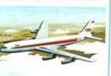
28. Convair 880 Length 129 ft. 4 in. Wingspan 120 ft. Height 36 ft. 4 in. Speed 615 m.p.h. Scale 1:400
