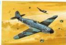
2. Messerschmitt ME 109 Length 29 ft. 4 in. Wingspan 32 ft. 6 in. Height 7 ft. 8 in. Speed 377 m.p.h. Scale 1:160
