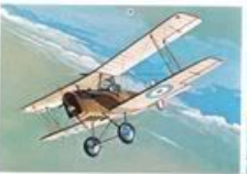
34. SE-5A Length ... 20 ft. 11 in. Wingspan ... 26 ft. 7 in. Height ... 9 ft. 6 in. Speed ... 126 m.p.h. Scale ... 1:100
