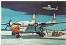
45. C-119 Flying Box Car Length ... 86 ft. 8 in. Wingspan 109 ft. 3 in. Height ... 26 ft. 3 in. Speed ... 296 m.p.h. Scale ... 1:260
