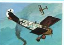
33. Fokker D-VII Length ... 22 ft. 9 in. Wingspan 29 ft. 3 1/2 in. Height ... 9 ft. 2 in. Speed ... 116 m.p.h. Scale ... 1:100
