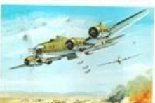
6. B-17 Flying Fortress Length 74 ft. 4 in. Wingspan 103 ft. 9 in. Height 19 ft. 3 in. Speed 300 m.p.h. Scale 1:250
