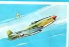
11. P-51 Mustang Length 32 ft. 3 in. Wingspan 37 ft. Height 37 ft. 8 in. Speed 437 m.p.h. Scale 1:150
