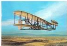
37. Kitty Hawk Length ... 19 ft. 9 in. Wingspan 40 ft. 4 in. Height ... 7 ft. 7 in. Speed ... 42 m.p.h. Scale ... 1:100
