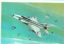
3. Russian MiG 21-C Length 47 ft. Wingspan 25 ft. Height 14 ft. 6 in. Speed 1,320 m.p.h. Scale 1:160
