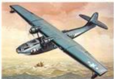
44. PBV-5A Catalina Length ... 65 ft. 2 in. Wingspan ... 104 ft. Height ... 20 ft. 2 in. Speed ... 179 m.p.h. Scale ... 1:340
