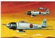
8. Japanese Zero-Zen Height ... 9 ft. 2 in. Length ... 29 ft. 5 in. Wingspan 36 ft. 1 in. Speed ... 346 m.p.h. Scale ..... 1:140
