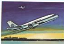
9. Boeing 707 Length 144 ft. 6 in. Wingspan 130 ft. 10 in. Height 42 ft. Speed 571 m.p.h. Scale 1:440
