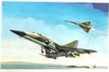
5. French Mirage 4A Length 77 ft. Wingspan 38 ft. 10 in. Height 18 ft. 6 in. Speed 1,454 m.p.h. Scale 1:260
