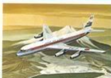
25. Douglas DC-8 Length ... 150 ft. 6 in. Wingspan 142 ft. 5 in. Height ... 42 ft. 6 in. Speed ... 580 m.p.h. Scale ... 1:150
