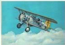
36. Boeing 74B-4 Length ... 20 ft. 4 1/2 in. Wingspan ... 30 ft. Height ... 9 ft. 9 in. Speed ... 184 m.p.h. Scale ... 1:100
