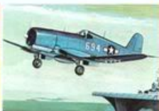
15. F4U Corsair Height ... 14 ft. 9 1/2 in. Length ... 33 ft. 8 1/2 in. Wingspan 40 ft. 11 1/2 in. Speed ... 425 m.p.h. Scale ..... 1:160
