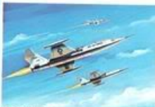
4. F-104 Starfighter Length 34 ft. 9 in. Wingspan 21 ft. 10 in. Height 13 ft. 6 in. Speed 1,450 m.p.h. Scale 1:220
