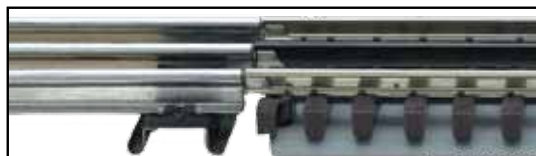
Use #6095 Tubular Transition Joiners. Shim the Atlas O track with 1/4" thick cork roadbed.
