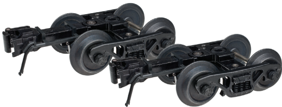
#66034 - 0 3 Rail - 70 Ton Roller Bearing Trucks
