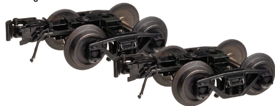
#66036 - 0 3 Rail - 70 Ton Modified Friction Bearing Trucks
