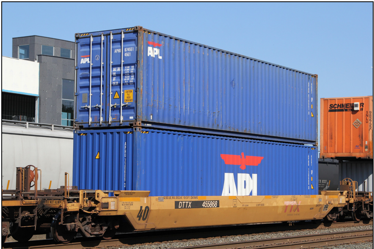
DTTX 455868 with two APL 40-foot high-cube container. Note the opposite end of the containers showing.
