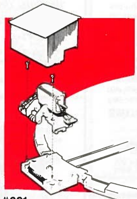
#301 TURNTABLE DRIVE UNIT
