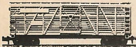
50' STAGGERED DOUBLE-DOOR BOXCAR
