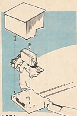
#301 TURNTABLE DRIVE UNIT
