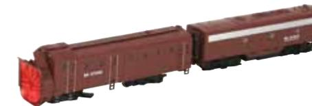
Burlington Northern employed plows to clear snowdrifts along the prairie lines. BN created a group of ten RSPUs, Rotary Snowplow Power Units, from retired F-series A and B units.
