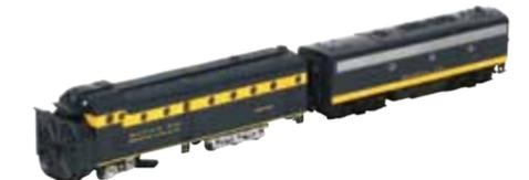
The Santa Fe plow was built in the Topeka shops from the rotary blades and housing of an 1892-built plow with traction motors, steel frame and car body. It too was built to clear prairie rails.
