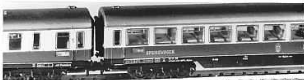
Close coupling in all Arnold rapido cars. Interior detail on TEE cars.
