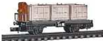
0456 Container Car Model of BTs 60 of the German Federal Railroad. Length 2". This car is used for the house to house service and carries three removable open containers. These are normally loaded with bulk goods. The containers are made of plastic and painted in silver. The platform railing is steel with a brakemen cabin.
